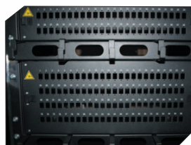
Possible installation of 19" and 21" devices
